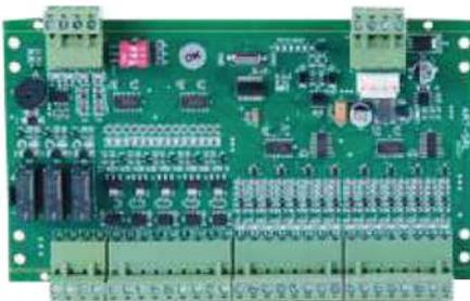
When parallel connection of the button to the ART-1 control panel is required, the SRL board is used as a CanBus converter. The SRL board allows parallel connections up to 16 floors and the connection of cabin buttons.
