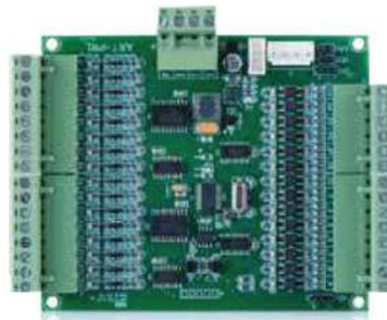
Series-parallel converter that transmits CanBus signals received from series buttons to control panel systems operating in parallel.
