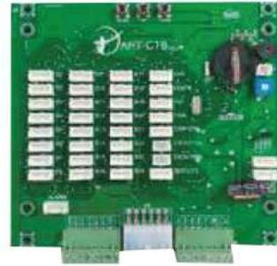
Thanks to CanBus communication, it transfers indicators, call buttons, and other cabin button components to the inspection box using a single cable.
